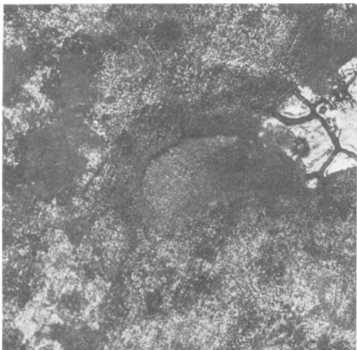
Fig. 34. Dissolution of Ni in the active potential range ( -0.85 V) in \text{Na}_2\text{SO}_4-15\% NaCl at 900^\circ\text{C} , in air, (E, Fig. 28). Surface ( \times 35 ).
