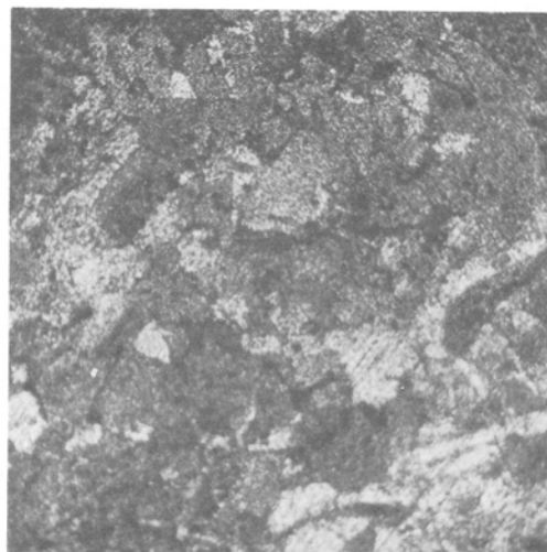
Fig. 35. Dissolution of Ni in the transpassive area ( -0.2 V) in \text{Na}_2\text{SO}_4-15\% NaCl at 900^\circ\text{C} , in air (F, Fig. 28). Surface ( \times 35 ).
